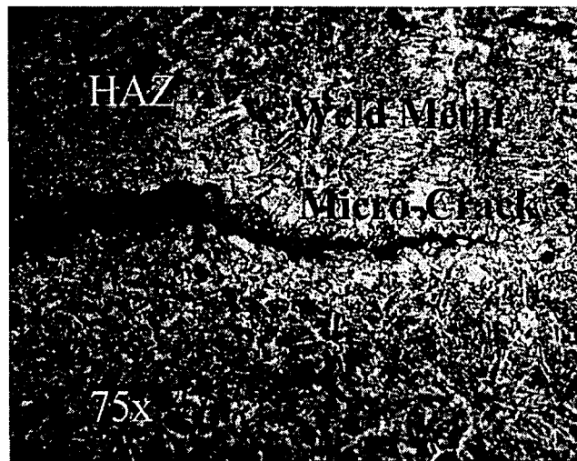
Figure 4.32: Micro-Cracking in Specimen 36-C2-Bottom-right Section
